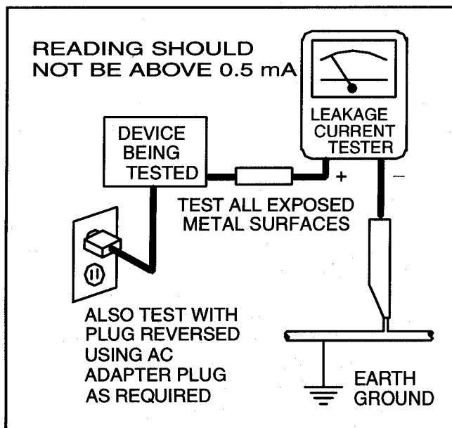
ANY MEASUREMENTS NOT WITHIN THE LIMITS SPECIFIED HEREIN INDICATE A POTENTIAL SHOCK HAZARD THAT MUST BE ELIMINATED BEFORE RETURNING THE INSTRUMENT TO THE CUSTOMER OR BEFORE CONNECTING THE ANTENNA OR ACCESSORIES.
