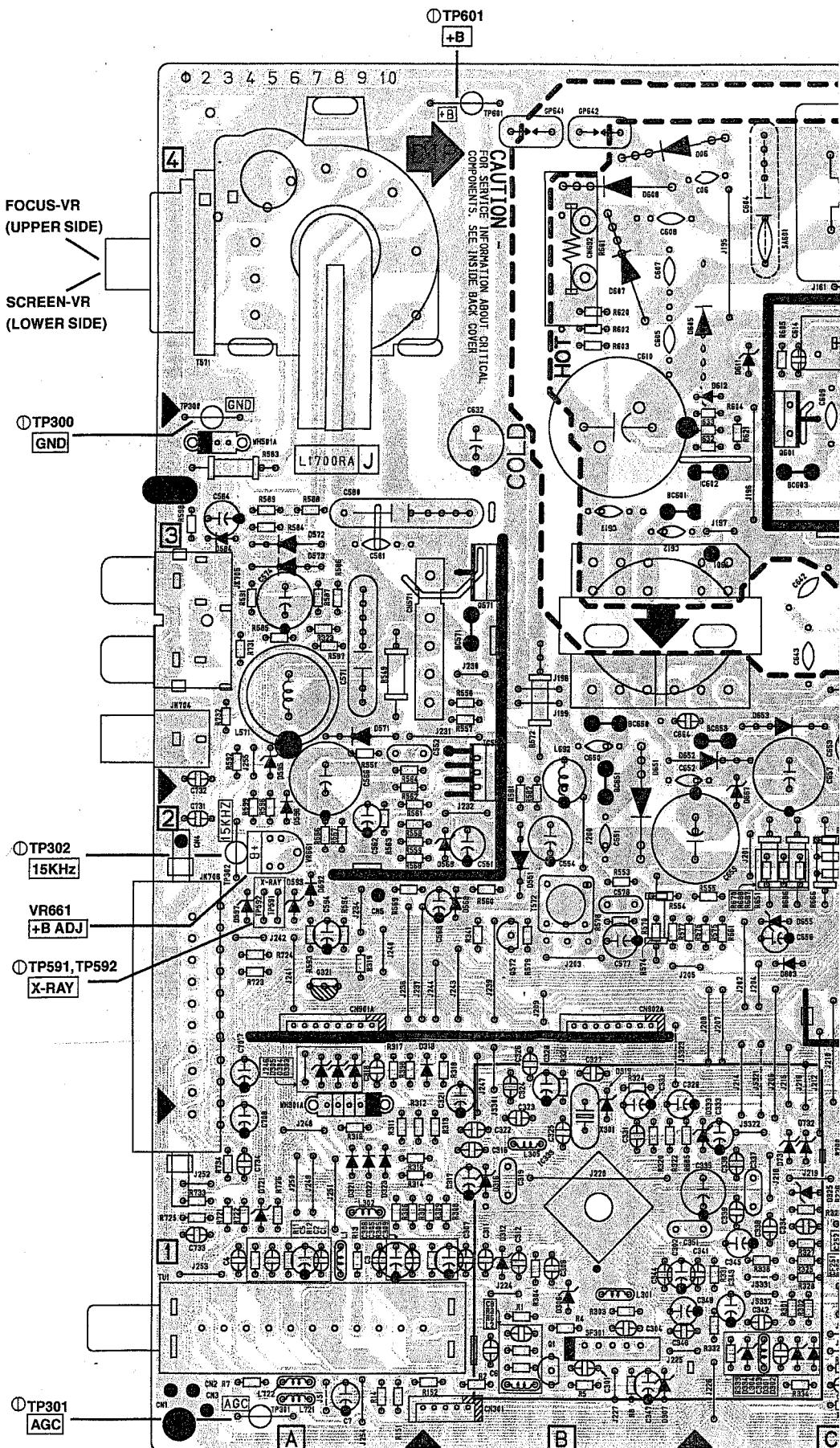
BECAUSE A HOT CHASSIS GROUND IS PRESENT IN THE POWER SUPPLY CIRCUIT, AN ISOLATION TRANSFORMER MUST BE USED. ALSO, IN ORDER TO HAVE THE ABILITY TO INCREASE THE INPUT SLOWLY, WHEN TROUBLESHOOTING THIS TYPE POWER SUPPLY CIRCUIT, A VARIABLE ISOLATION TRANSFORMER IS REQUIRED.
