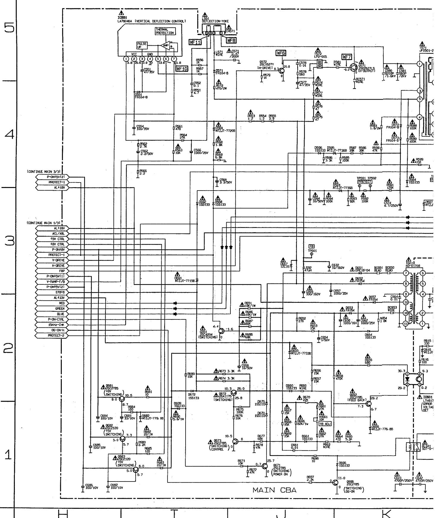
BECAUSE A HOT CHASSIS GROUND IS PRESENT IN THE POWER SUPPLY CIRCUIT, AN ISOLATION TRANSFORMER MUST BE USED. ALSO, IN ORDER TO HAVE THE ABILITY TO INCREASE THE INPUT SLOWLY, WHEN TROUBLESHOOTING THIS TYPE POWER SUPPLY CIRCUIT, A VARIABLE ISOLATION TRANSFORMER IS REQUIRED.
