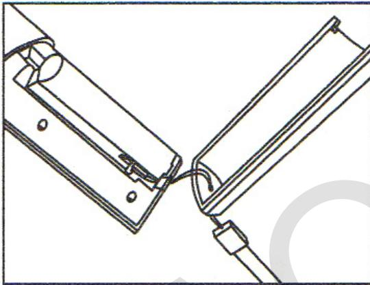
1. Pull the strap loop through the hole at the bottom of a battery compartment;
